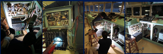
CPP control unit trouble shooting repair ( Sagita)
